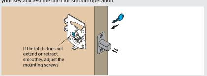
Secure the mounting plate with the mounting screws.
