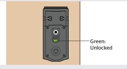
If the Status LED is displaying the wrong lock status, flip switch #4.
